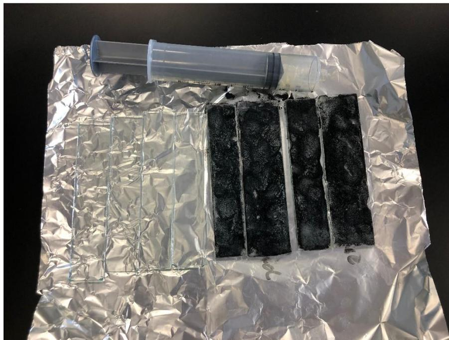
Figure 8. Applied functionalized SIG stationary phase on a glass.
