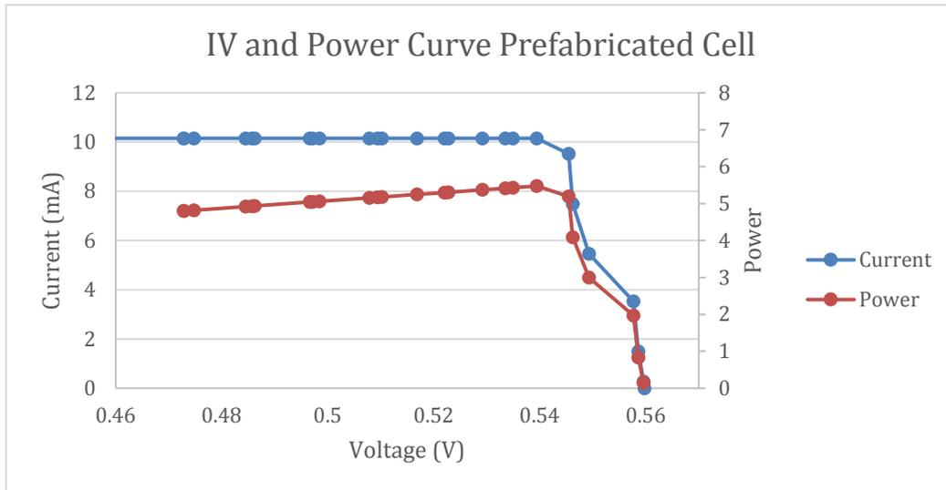
Figure 53: Prefabricated silicon solar cell tested with a 1.0 Ohm resistor and a maximum current draw of 10.0 mA.
