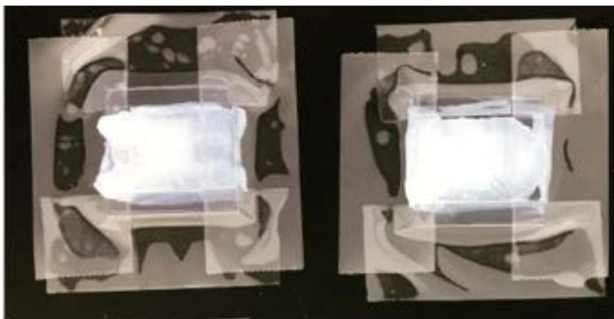
*Figure 7: Glass slides with tape creating the well for the  $\text{TiO}_2$  nanoparticle layer.*
