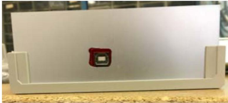
*Figure 23: Back Panel of the Instrument: The USB cord from the DAQ Board comes out of the back panel of the instrument and inserts into the computer to power and drive the DAQ board.*
