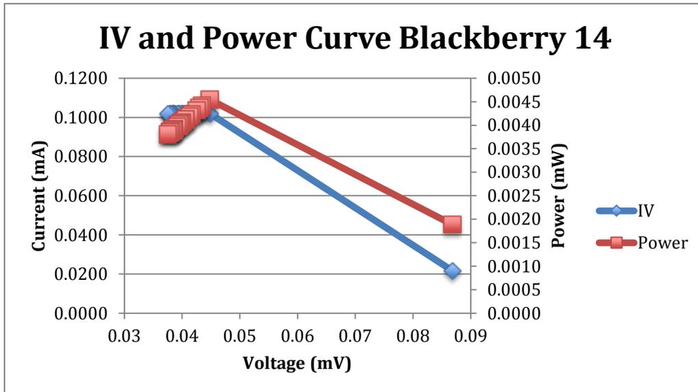
Figure 57: DSSC Blackberry #14 fabricated with the ferrocene electrolyte and blackberry dye. The 100,000 Ohm resistor was used and 0.5 mA was set as the maximum current draw.
