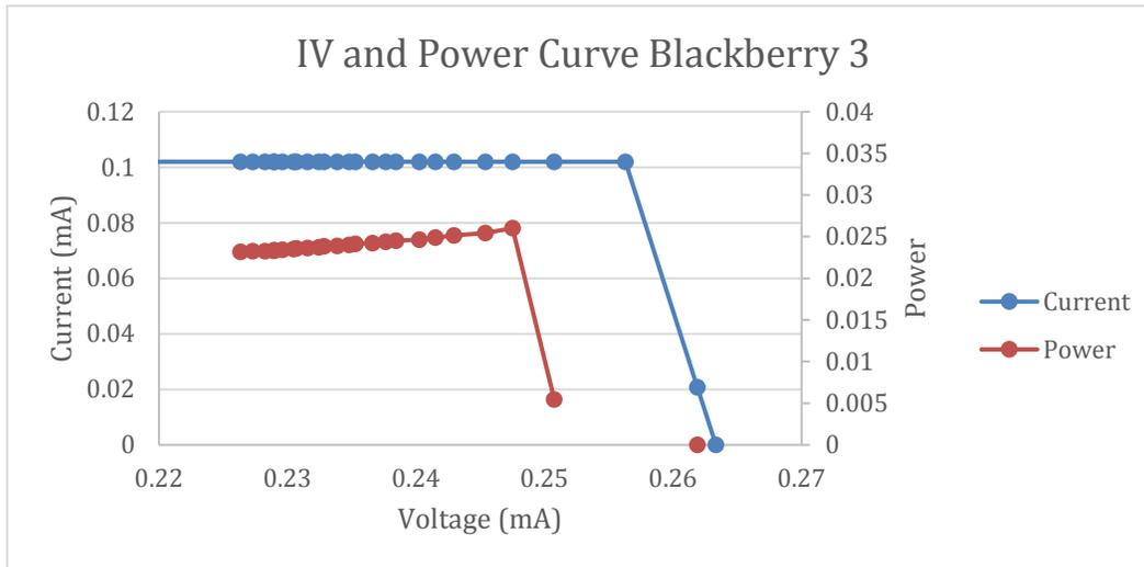
Figure 45: DSSC Blackberry #3 fabricated with the iodine electrolyte and blackberry dye. The 100,000 Ohm resistor was used and 0.5 mA was set as the maximum current draw.
