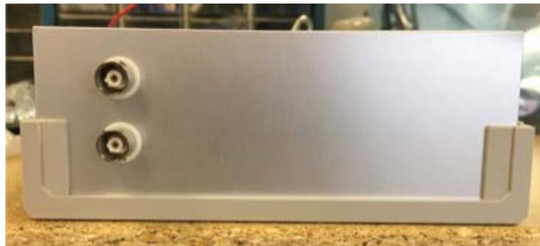
*Figure 24: Front Panel of the Instrument: Two alligator clips soldered to wires attach to the BNC connectors on this front panel and go to the solar cell.*
