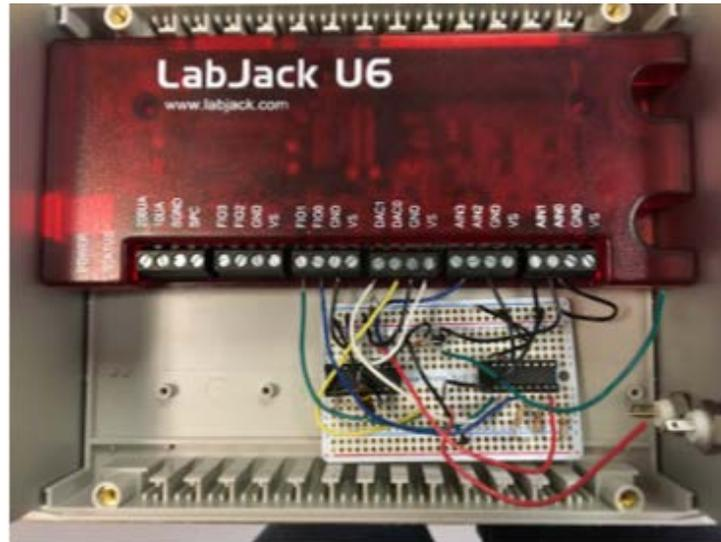
*Figure 25: DAQ Board and Circuit: The circuit connects to the DAQ board and to the solar cell by way of alligator clips. These are the main electrical components of the new instrument and allow the IV curve to be created.*
