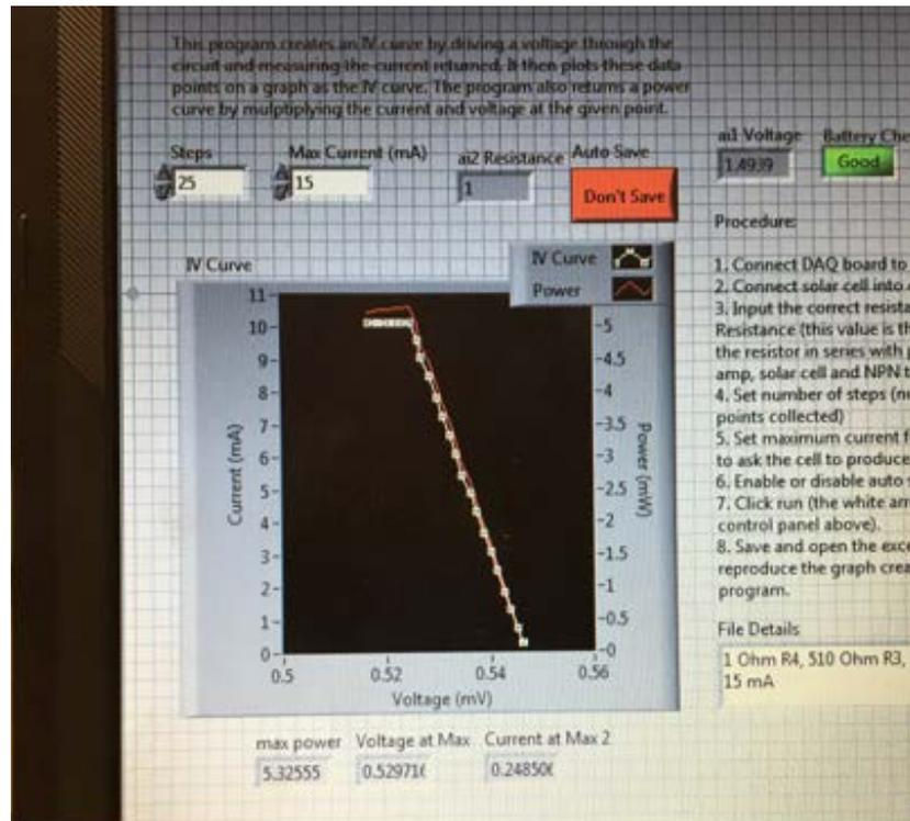
Figure 22: IV and Power curve returned by the instrument on the front panel of the LabView program
