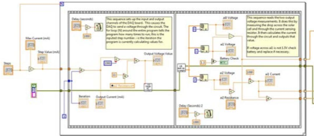
Figure 19: Block Diagram 1 showing the first part of the computer program designed for the instrument.
