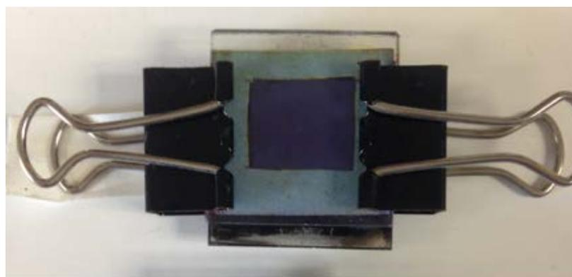
*Figure 13: Fully assembled DSSC held together with binder clips to create a tight seal around the gasket to hold the electrolyte in the well.*
