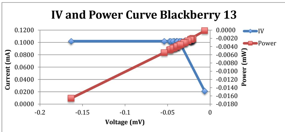
Figure 56: DSSC Blackberry #13 fabricated with the ferrocene electrolyte and blackberry dye. The 100,000 Ohm resistor was used and 0.5 mA was set as the maximum current draw.
