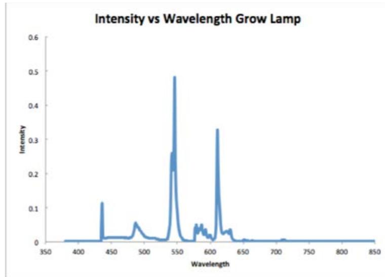
Figure 36: Emission Spectrum of the plant grow lamp with three distinct peaks.
