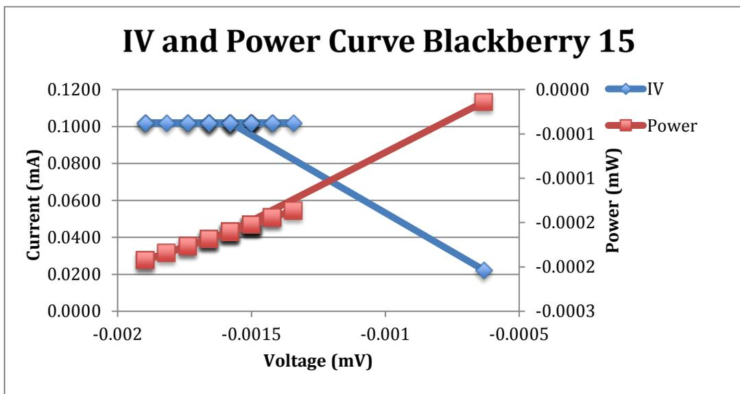
Figure 58 : DSSC Blackberry #15 fabricated with the ferrocene electrolyte and blackberry dye. The 100,000 Ohm resistor was used and 0.5 mA was set as the maximum current draw.
