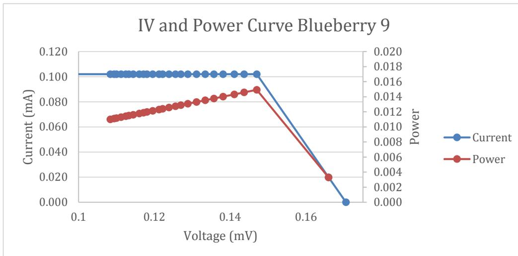
Figure 51: DSSC Blueberry #9 fabricated with the iodine electrolyte and blueberry dye. The 100,000 Ohm resistor was used and 0.5 mA was set as the maximum current draw.
