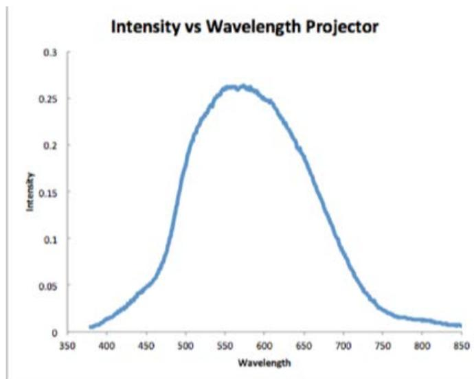
Figure 37: Emission Spectrum of the overhead projector lamp, with a smooth curve.
