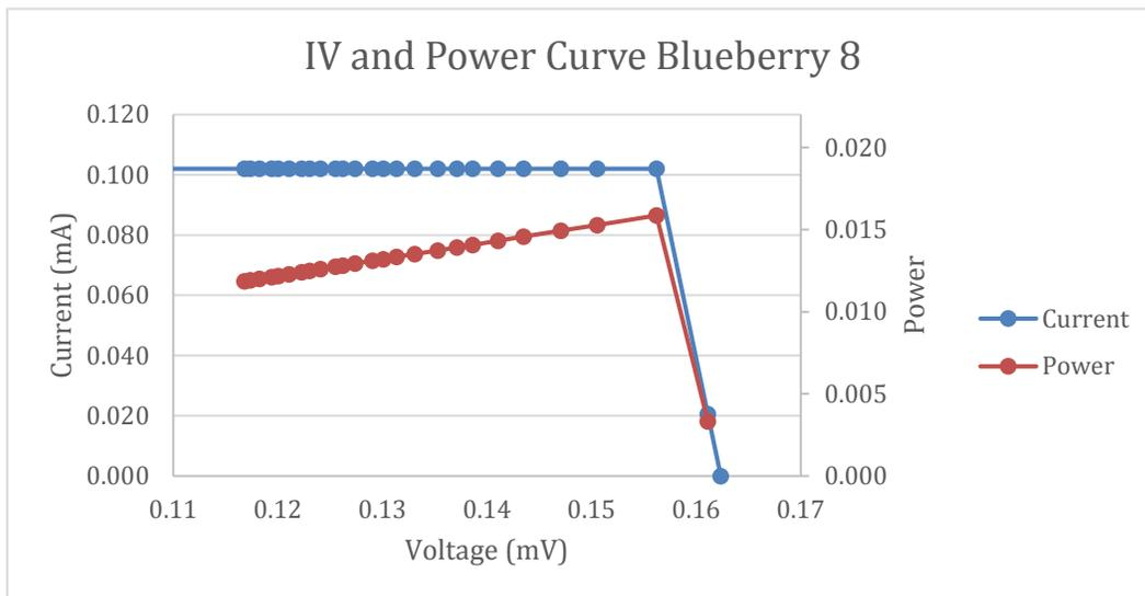
Figure 50: DSSC Blueberry #8 fabricated with the iodine electrolyte and blueberry dye. The 100,000 Ohm resistor was used and 0.5 mA was set as the maximum current draw.
