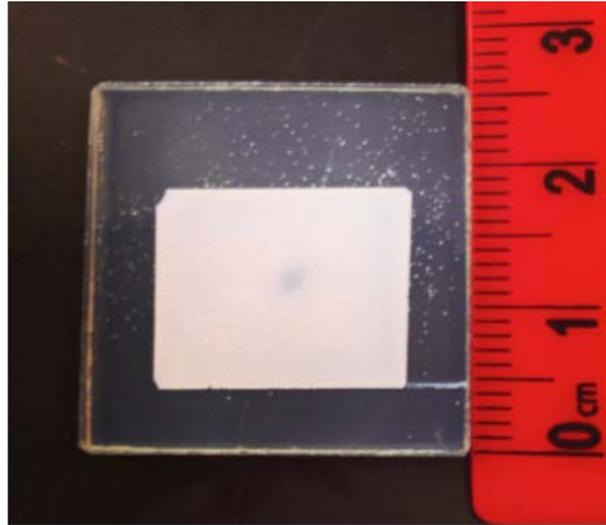
*Figure 8: Titanium Dioxide Cathode: Titanium dioxide nanoparticle coated conductive glass slides ready to be stained and assembled into a functioning solar cell.*
