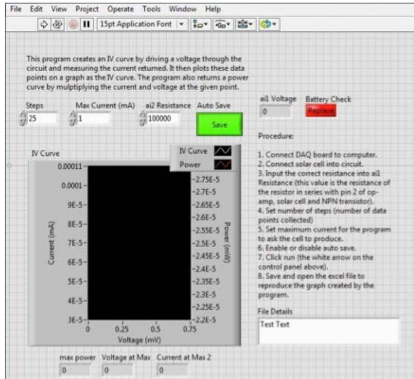
Figure 21: Front Panel of the instrument, where the original IV and Power curves appear.
