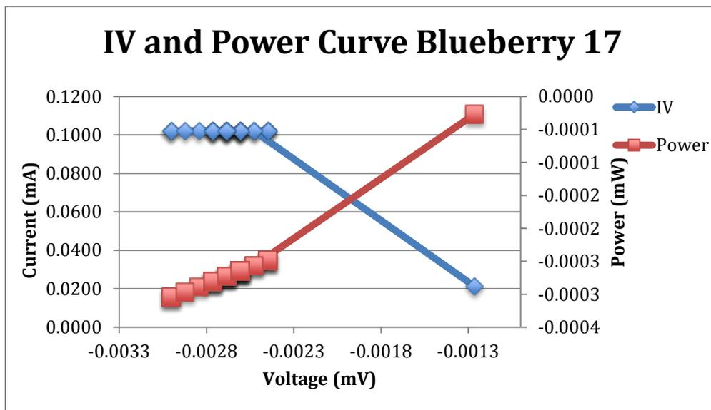
Figure 60: DSSC Blueberry #17 fabricated with the ferrocene electrolyte and blueberry dye. The 100,000 Ohm resistor was used and 0.5 mA was set as the maximum current draw.
