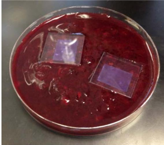
*Figure 10: Titanium dioxide glass slides being stained with crushed blackberry juice.*
