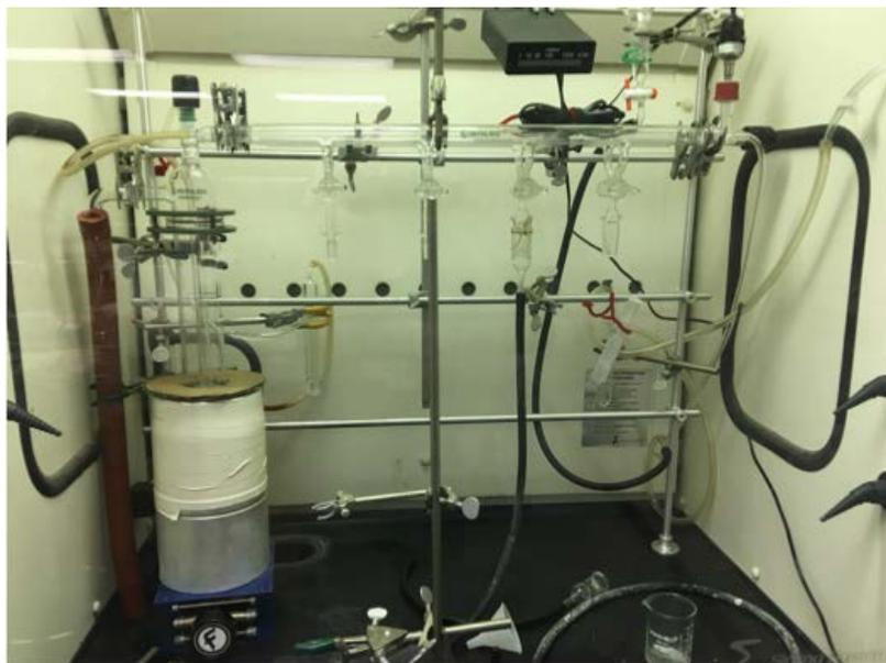
*Figure 17: Schlenk line used to bubble Nitrogen through the ferrocene electrolyte after synthesis*
