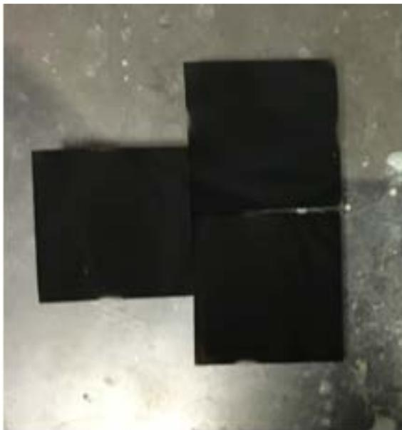
*Figure 9: Solar Cell Anode: Carbon coated conductive glass slides ready to be assembled into a functioning solar cell to act as the counter electrode in the circuit.*
