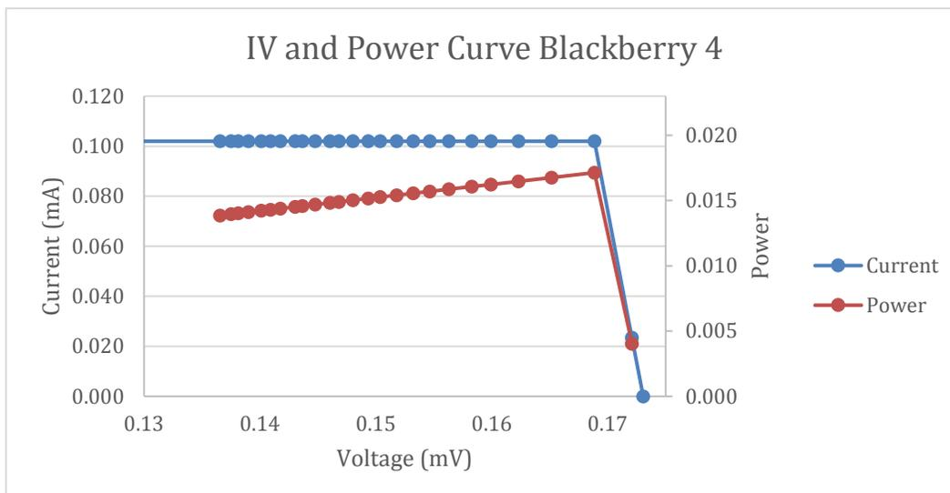
Figure 46: DSSC Blackberry #4 fabricated with the iodine electrolyte and blackberry dye. The 100,000 Ohm resistor was used and 0.5 mA was set as the maximum current draw.
