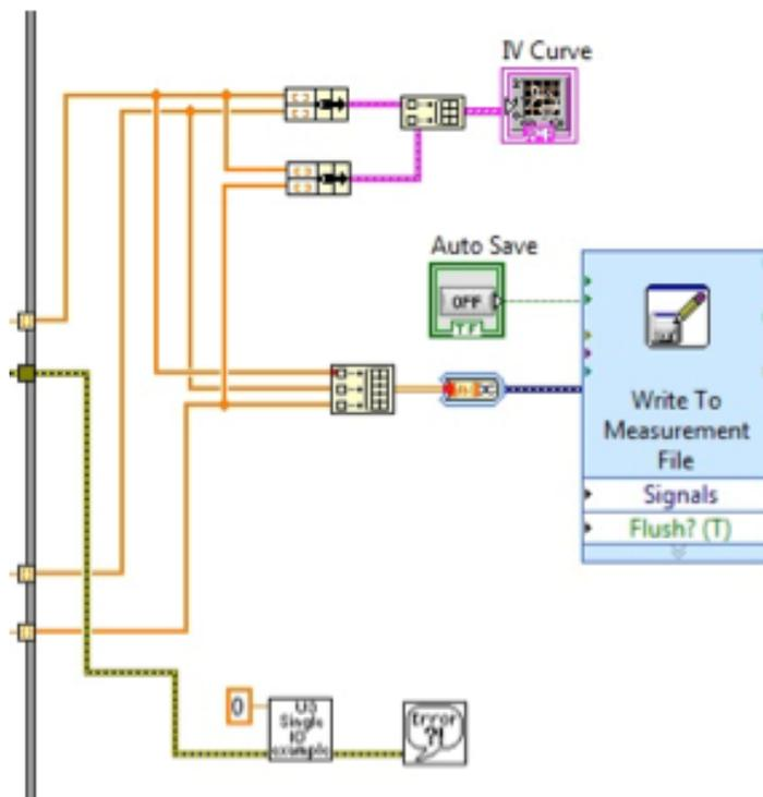
Figure 20: Block Diagram 2 showing the second part of the computer program designed for the instrument, this part writes the graph files.
