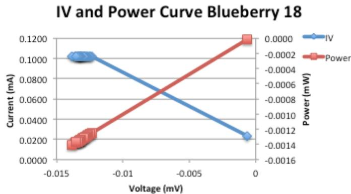
Figure 42: DSSC Blueberry #18 fabricated with the ferrocene electrolyte and blueberry dye. The 100,000 Ohm resistor was used and 0.5 mA was set as the maximum current draw.
