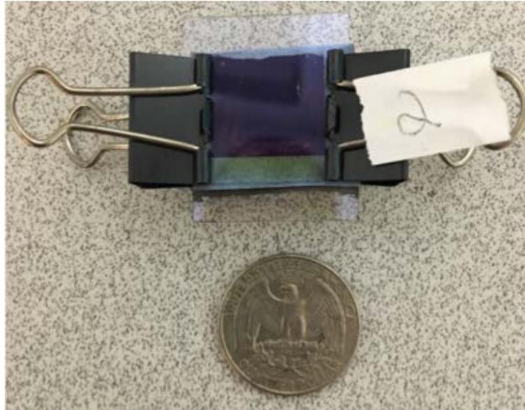
*Figure 33: Fully assembled DSSC made with the new glass slides. The glass is clear, clean and easy to wipe clean to make a good connection with the alligator clips.*
