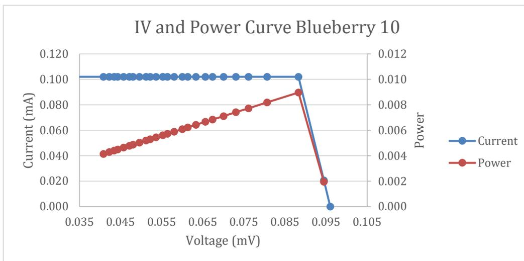
Figure 52: DSSC Blueberry #10 fabricated with the iodine electrolyte and blueberry dye. The 100,000 Ohm resistor was used and 0.5 mA was set as the maximum current draw.
