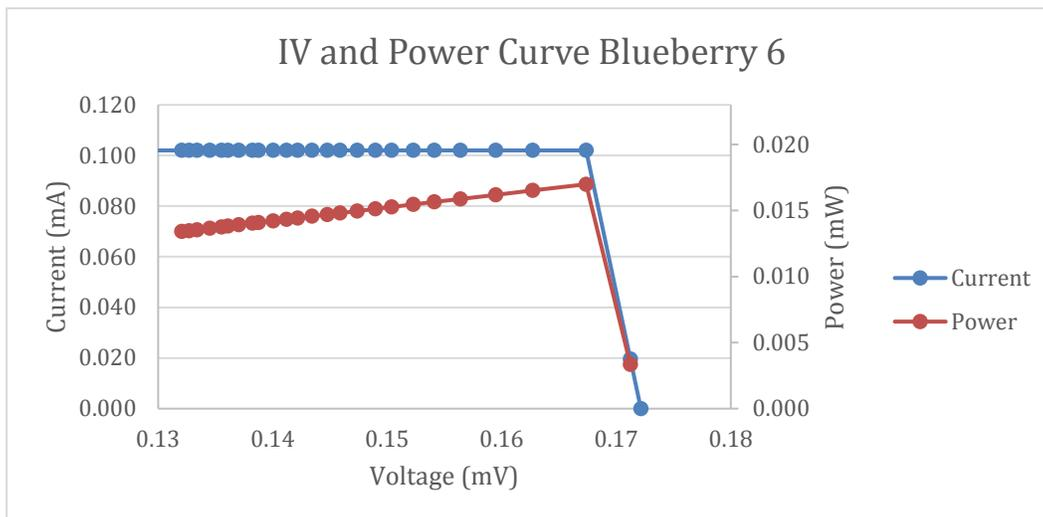
*Figure 48: DSSC Blueberry #6 fabricated with the iodine electrolyte and blueberry dye. The 100,000 Ohm resistor was used and 0.5 mA was set as the maximum current draw.*
