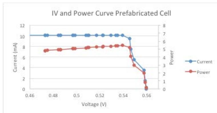
Figure 38: Prefabricated silicon solar cell tested with a 1.0 Ohm resistor and a maximum current draw of 10.0 mA.
