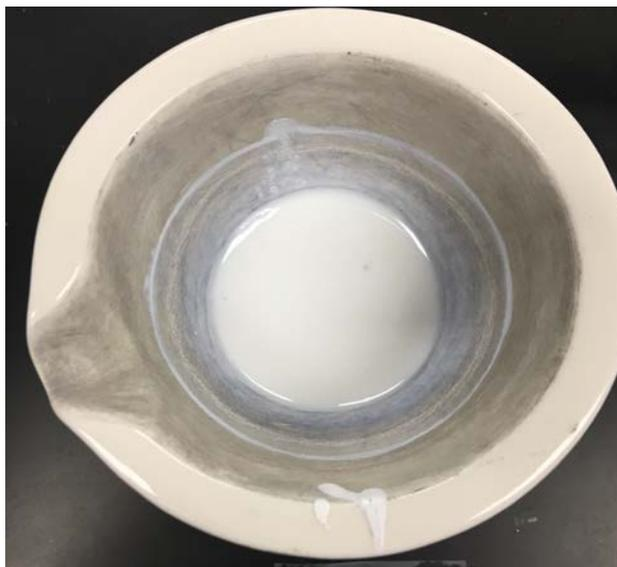
*Figure 6: Titanium Dioxide, trimesic acid, and water that has been ground together with a mortar and pestle.*
