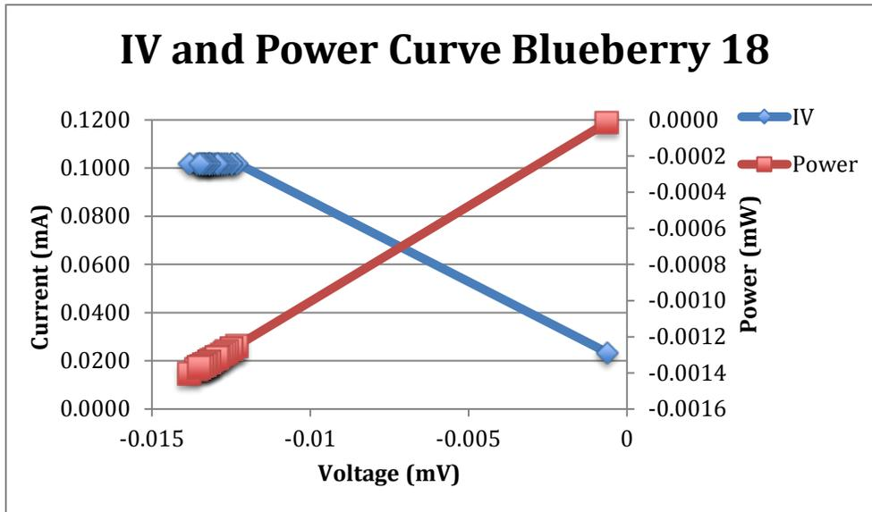
Figure 61: DSSC Blueberry #18 fabricated with the ferrocene electrolyte and blueberry dye. The 100,000 Ohm resistor was used and 0.5 mA was set as the maximum current draw.
