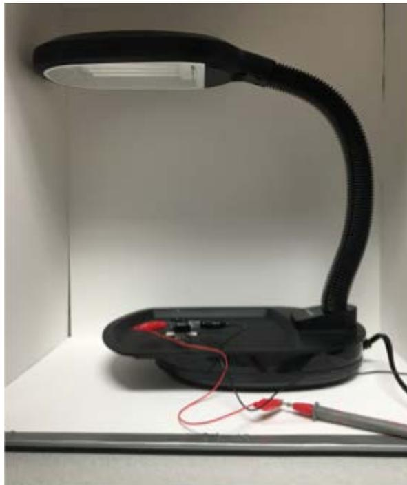
*Figure 31: Test Method 1: The grow lamp and light containment box previously used to test the solar cells.*
