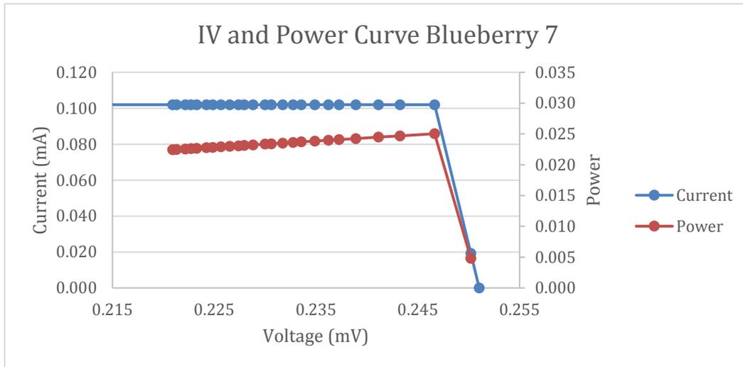
Figure 49: DSSC Blueberry #7 fabricated with the iodine electrolyte and blueberry dye. The 100,000 Ohm resistor was used and 0.5 mA was set as the maximum current draw.
