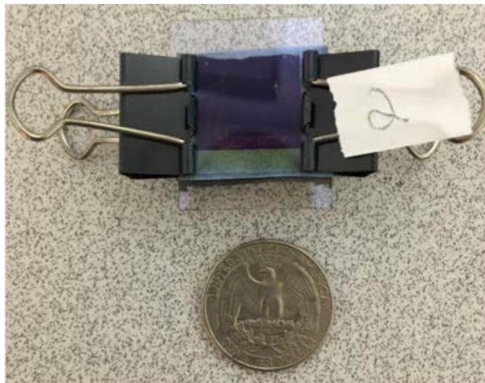
*Figure 4: Natural Dye Sensitized (DSSC) solar cell fabricated in lab with a quarter to show size*
