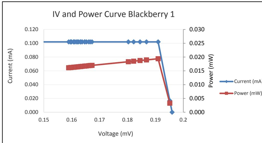
Figure 43: DSSC Blackberry #1 fabricated with the iodine electrolyte and blackberry dye. The 100,000 Ohm resistor was used and 0.5 mA was set as the maximum current draw.
