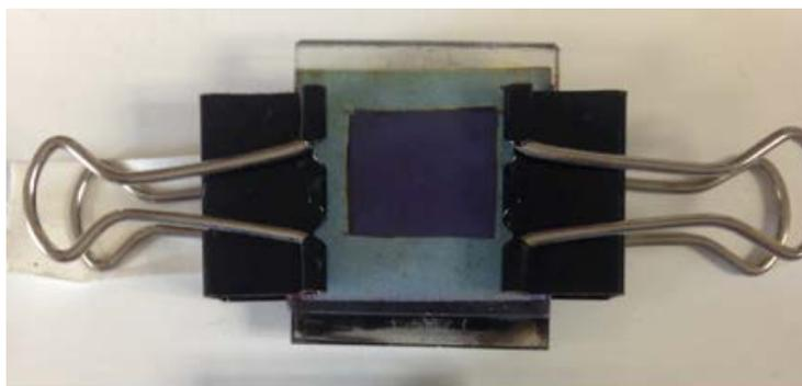
*Figure 32: Fully assembled DSSC made with the old glass slides. The glass is cloudy, dirty, and difficult to clean after trials and to make good connections with the alligator clips.*
