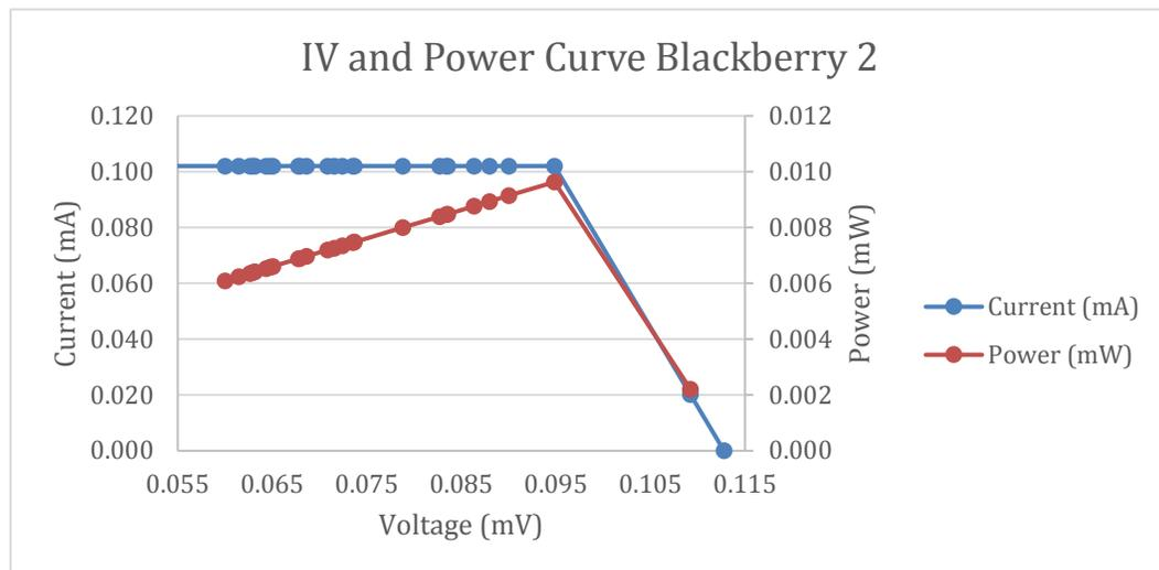
Figure 44: DSSC Blackberry #2 fabricated with the iodine electrolyte and blackberry dye. The 100,000 Ohm resistor was used and 0.5 mA was set as the maximum current draw.
