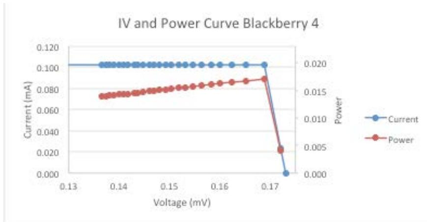
Figure 39: DSSC Blackberry #4 fabricated with the iodine electrolyte and blackberry dye. The 100,000 Ohm resistor was used and 0.5 mA was set as the maximum current draw.
