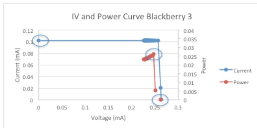
*Figure 1: IV and Power Curve where short-circuit current is shown crossing the y-axis, open-circuit current crossing the x-axis, and maximum power being y-max.*
