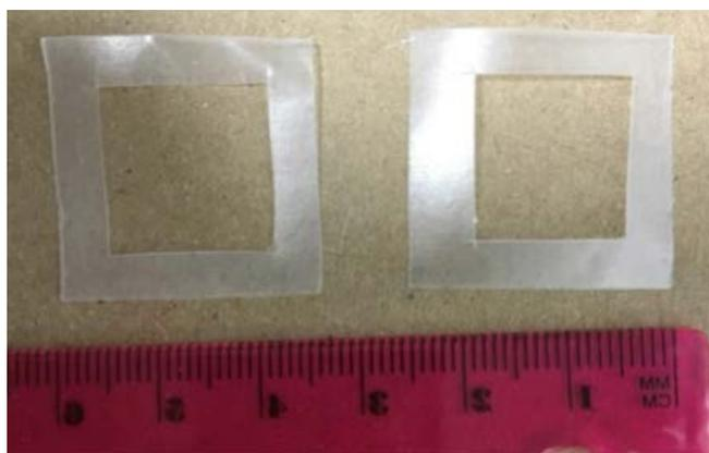
*Figure 29: Parafilm Gasket: Two pieces of parafilm gasket cut to fit the solar cell and create the well for the electrolyte.*
