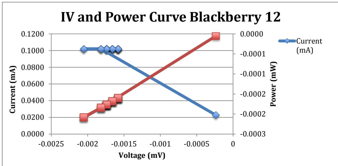
Figure 55: DSSC Blackberry #12 fabricated with the ferrocene electrolyte and blackberry dye. The 100,000 Ohm resistor was used and 0.5 mA was set as the maximum current draw.
