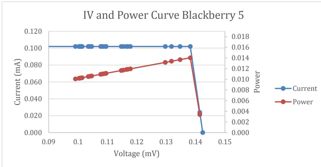
*Figure 47: DSSC Blackberry #5 fabricated with the iodine electrolyte and blackberry dye. The 100,000 Ohm resistor was used and 0.5 mA was set as the maximum current draw.*
