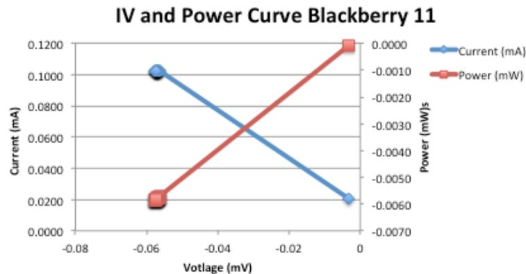
Figure 41: DSSC Blackberry#11 fabricated with the ferrocene electrolyte and blackberry dye. The 100,000 Ohm resistor was used and 0.5 mA was set as the maximum current draw.
