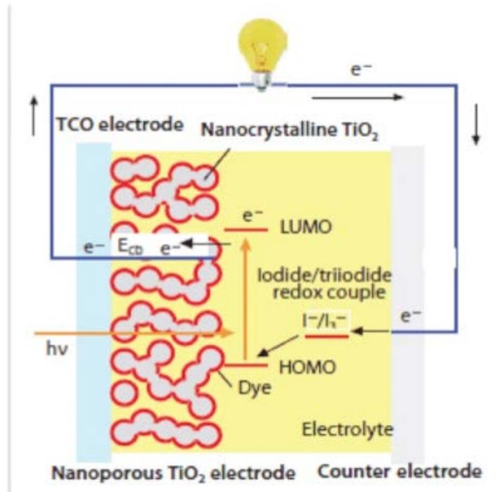
Figure 5: Solar Cell Electron Diagram: An electron from the dye is promoted and flows through the nanoparticle layer, through the conductive glass and through a wire before returning to the counter electrode and entering an oxidation-reduction reaction in the electrolyte.<sup>11</sup>
