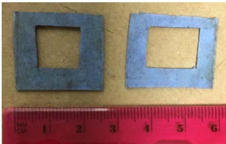
*Figure 30: Garlock Gasket: Two pieces of PTFE Blue Gylon 3504 gasket cut to the same dimension as the area of the titanium dioxide layer on the inner side and slightly smaller than the dimensions of the glass slide on the outer side.*
