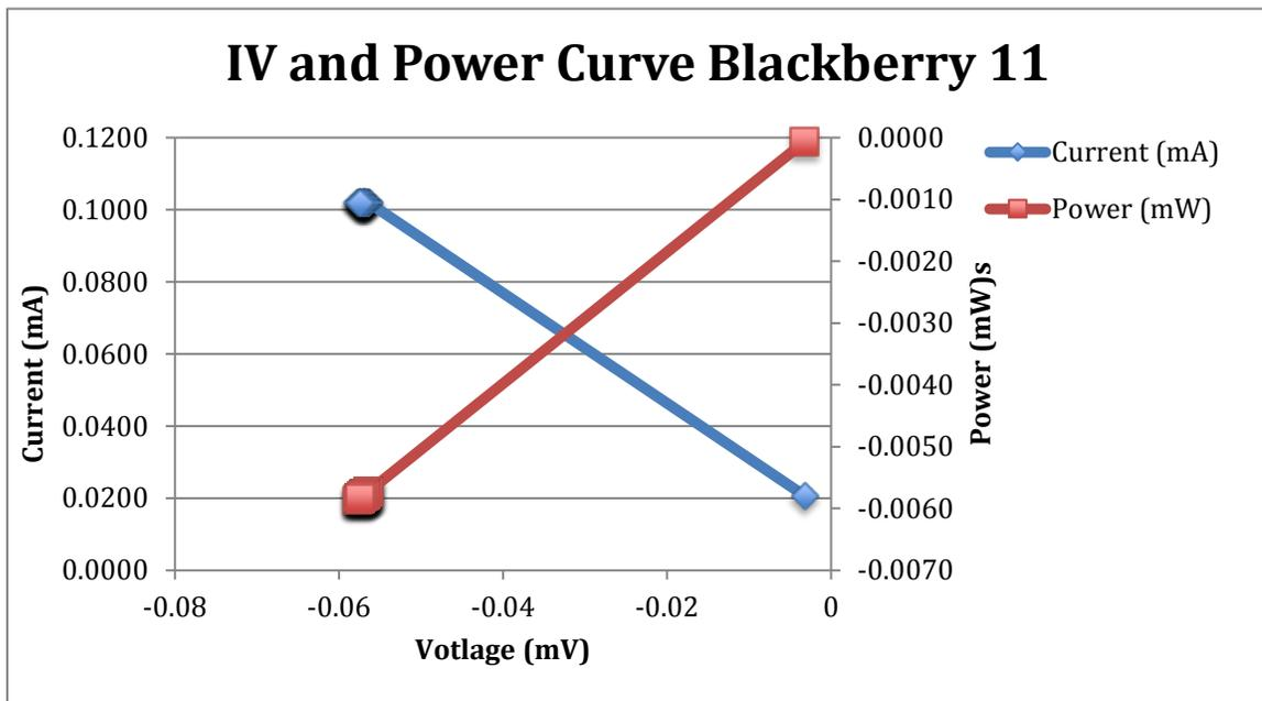
Figure 54: DSSC Blackberry#11 fabricated with the ferrocene electrolyte and blackberry dye. The 100,000 Ohm resistor was used and 0.5 mA was set as the maximum current draw.
