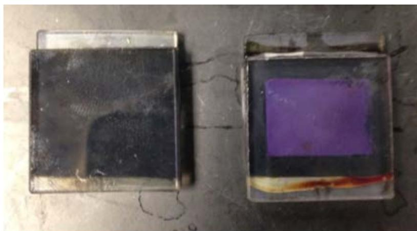
*Figure 12: Fully Assembled Solar Cell: On the left is the anode, the carbon coated slide. On the right is the cathode, the dye stained titanium dioxide coated slide. When put together with the electrolyte these two slides form a fully functioning solar cell.*
