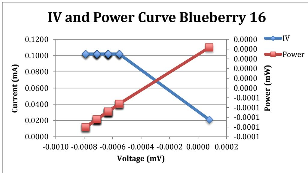
Figure 59: DSSC Blueberry #16 fabricated with the ferrocene electrolyte and blueberry dye. The 100,000 Ohm resistor was used and 0.5 mA was set as the maximum current draw.
