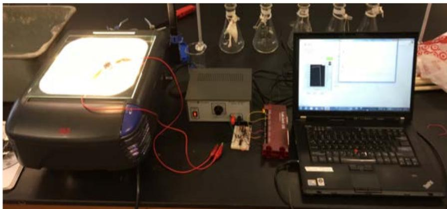
Figure 27: Instrument set up for testing DSSCs using the computer program, circuit and overhead projector
