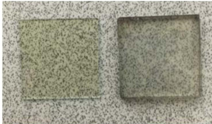
*Figure 34: Glass Slides: On the right is the old glass used in cell fabrication. It became stained and difficult to clean so new glass was bought for future trials (glass slide on the left).*
