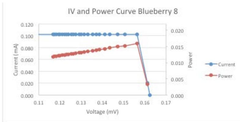
Figure 40: DSSC Blueberry #8 fabricated with the iodine electrolyte and blueberry dye. The 100,000 Ohm resistor was used and 0.5 mA was set as the maximum current draw.
