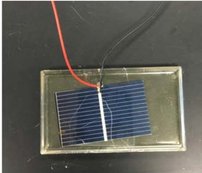
*Figure 3: Silicon prefabricated solar cell used as the control for testing the instrument and as a comparison to DSSCs prepared in-house.*
