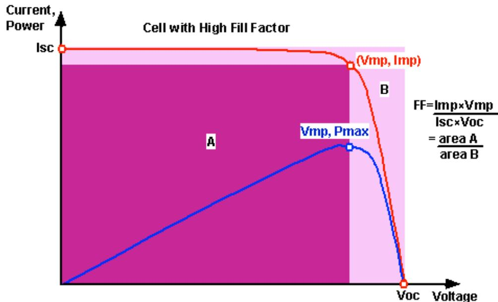
Figure 2: Graph showing how to calculate fill factor. Area A is determined by multiplying the current and voltage at the maximum power point and Area B is determined by multiplying the open circuit current and voltage. Fill Factor is the ration between the two.<sup>7</sup>
