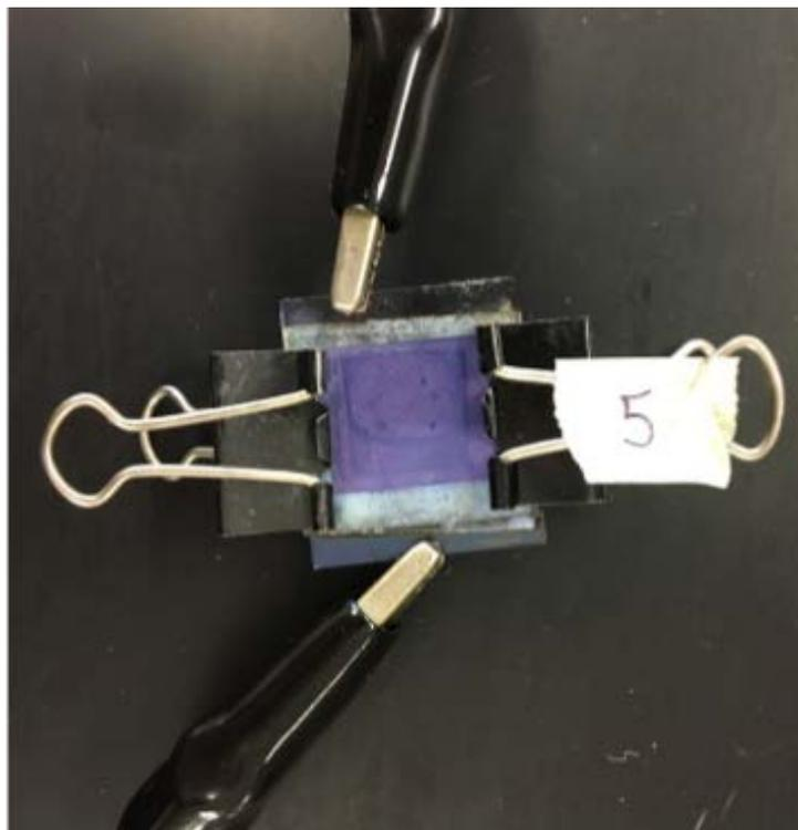
*Figure 26: Instrument wires connected to solar cell to complete the circuit and allow the instrument to collect data*
